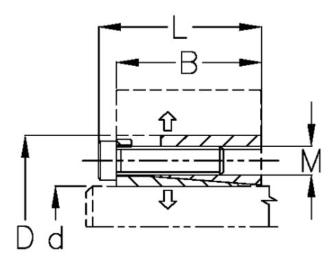
$\begin{array}{lll} \text{B mm} & = 33.5 \\ \text{d H8 mm} & = 65 \\ \text{D mm} & = 95 \\ \text{Fit tolerance} & = \text{Aksel h8, Nav H8} \\ \text{F kN torque} & = 105 \\ \text{L mm} & = 41 \\ \text{M mm} & = \text{M8} \\ \text{P N/mm2 surface pressure on shaft/hub} = 150 \\ \end{array}$
